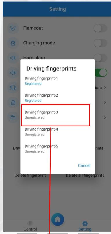
Step 2: Choose an unregistered slot to register new fingerprint
